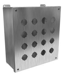
Hammond pushbutton enclosure, 16 holes, 30mm, NEMA 4/4X, 12 x 11 x 5in (HxWxD), wall mount, 304 stainless steel, #4 brush finish, hinged screw cover.
