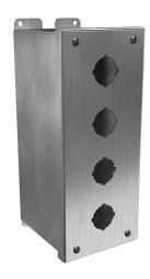
Hammond pushbutton enclosure, 4 holes, 30mm, NEMA 4/4X,  $10 \times 4 \times 5$ in (HxWxD), wall mount, 304 stainless steel, #4 brush finish, hinged screw cover.
