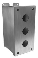
Hammond pushbutton enclosure, 3 holes, 30mm, NEMA 4/4X, 8 x 4 x 5in (HxWxD), wall mount, 304 stainless steel, #4 brush finish, hinged screw cover.
