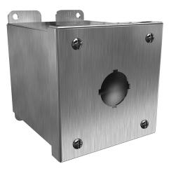
Hammond pushbutton enclosure, 1 hole, 30mm, NEMA 4/4X, 4 x 4 x 5in (HxWxD), wall mount, 304 stainless steel, #4 brush finish, screw cover.
