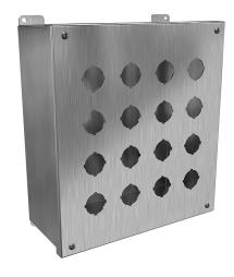
Hammond pushbutton enclosure, 16 holes, 30mm, NEMA 4/4X,  $12 \times 11 \times 5$  in (HxWxD), wall mount, 316 stainless steel, #4 brush finish, hinged screw cover.
