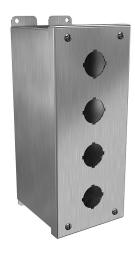
Hammond pushbutton enclosure, 4 holes, 30mm, NEMA 4/4X,  $10 \times 4 \times 5$  in (HxWxD), wall mount, 316 stainless steel, #4 brush finish, hinged screw cover.
