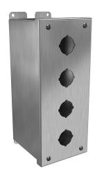
Hammond pushbutton enclosure, 4 holes, 30mm, NEMA 4/4X, 10 x 4 x 5in (HxWxD), wall mount, 316 stainless steel, #4 brush finish, hinged screw cover.
