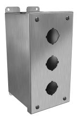
Hammond pushbutton enclosure, 3 holes, 30mm, NEMA 4/4X, 8 x 4 x 5in (HxWxD), wall mount, 316 stainless steel, #4 brush finish, hinged screw cover.
