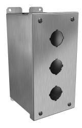
Hammond pushbutton enclosure, 3 holes, 30mm, NEMA 4/4X, 8  $\times$  4  $\times$  5in (HxWxD), wall mount, 316 stainless steel, #4 brush finish, hinged screw cover.
