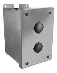
Hammond pushbutton enclosure, 2 holes, 30mm, NEMA 4/4X, 6 x 4 x 5in (HxWxD), wall mount, 316 stainless steel, #4 brush finish, hinged screw cover.
