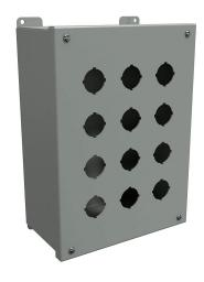
Hammond pushbutton enclosure, 12 holes, 30mm, NEMA 12/13, 12 x 9 x 5in (HxWxD), wall mount, carbon steel, ANSI 61 gray, powder coat finish, hinged screw cover.
