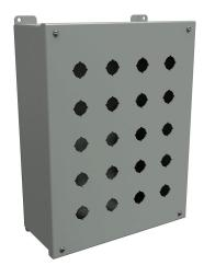
Hammond pushbutton enclosure, 20 holes, 22mm, NEMA 12/13, 14 x 11 x 5in (HxWxD), wall mount, carbon steel, ANSI 61 gray, powder coat finish, hinged screw cover.
