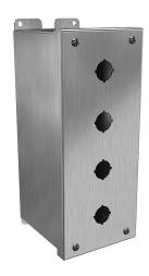
Hammond pushbutton enclosure, 4 holes, 22mm, NEMA 4/4X, 10 x 4 x 5in (HxWxD), wall mount, 316 stainless steel, #4 brush finish, hinged screw cover.
