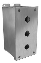
Hammond pushbutton enclosure, 3 holes, 22mm, NEMA 4/4X, 8 x 4 x 5in (HxWxD), wall mount, 316 stainless steel, #4 brush finish, hinged screw cover.
