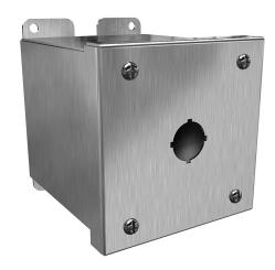
Hammond pushbutton enclosure, 1 hole, 22mm, NEMA 4/4X, 4 x 4 x 5in (HxWxD), wall mount, 316 stainless steel, #4 brush finish, screw cover.
