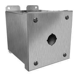
Hammond pushbutton enclosure, 1 hole, 22mm, NEMA 4/4X, 4  $\times$  4  $\times$  5in (HxWxD), wall mount, 316 stainless steel, #4 brush finish, screw cover.
