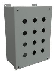
Hammond pushbutton enclosure, 12 holes, 22mm, NEMA 12/13, 12 x 9 x 5in (HxWxD), wall mount, carbon steel, ANSI 61 gray, powder coat finish, hinged screw cover.
