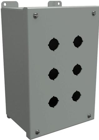
Hammond pushbutton enclosure, 6 holes, 22mm, NEMA 12/13, 10 x 7 x 5in (HxWxD), wall mount, carbon steel, ANSI 61 gray, powder coat finish, hinged screw cover.
