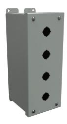
Hammond pushbutton enclosure, 4 holes, 22mm, NEMA 12/13, 10 x 4 x 5in (HxWxD), wall mount, carbon steel, ANSI 61 gray, powder coat finish, hinged screw cover.
