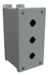
Hammond pushbutton enclosure, 3 holes, 22mm, NEMA 12/13, 8 x 4 x 5in (HxWxD), wall mount, carbon steel, ANSI 61 gray, powder coat finish, hinged screw cover.
