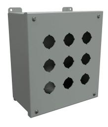
Hammond pushbutton enclosure, 9 holes, 30mm, NEMA 12/13, 10 x 9 x 5in (HxWxD), wall mount, carbon steel, ANSI 61 gray, powder coat finish, hinged screw cover.
