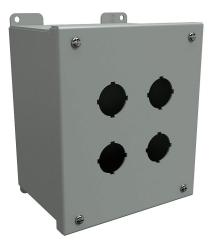
Hammond pushbutton enclosure, 4 holes, 30mm, NEMA 12/13, 8 x 7 x 5in (HxWxD), wall mount, carbon steel, ANSI 61 gray, powder coat finish, hinged screw cover.
