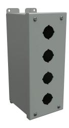
Hammond pushbutton enclosure, 4 holes, 30mm, NEMA 12/13, 10 x 4 x 5in (HxWxD), wall mount, carbon steel, ANSI 61 gray, powder coat finish, hinged screw cover.
