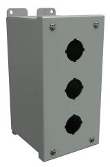
Hammond pushbutton enclosure, 3 holes, 30mm, NEMA 12/13, 8 x 4 x 5in (HxWxD), wall mount, carbon steel, ANSI 61 gray, powder coat finish, hinged screw cover.
