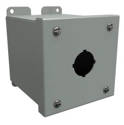
Hammond pushbutton enclosure, 1 hole, 30mm, NEMA 12/13, 4 x 4 x 5in (HxWxD), wall mount, carbon steel, ANSI 61 gray, powder coat finish, screw cover.
