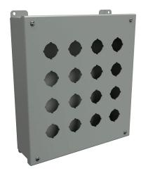
Hammond pushbutton enclosure, 16 holes, 30mm, NEMA 12/13, 12 x 11 x 3in (HxWxD), wall mount, carbon steel, ANSI 61 gray, powder coat finish, hinged screw cover.
