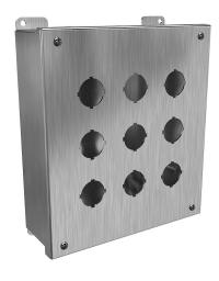
Hammond pushbutton enclosure, 9 holes, 30mm, NEMA 3R/4/4X,  $10 \times 9 \times 3$ in (HxWxD), wall mount, 304 stainless steel, #4 brush finish, hinged screw cover.
