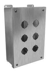
Hammond pushbutton enclosure, 6 holes, 30mm, NEMA 3R/4/4X,  $10 \times 7 \times 3$ in (HxWxD), wall mount, 304 stainless steel, #4 brush finish, hinged screw cover.
