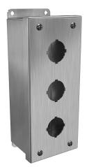
Hammond pushbutton enclosure, 3 holes, 30mm, NEMA 3R/4/4X, 8 x 4 x 3in (HxWxD), wall mount, 304 stainless steel, #4 brush finish, screw cover.
