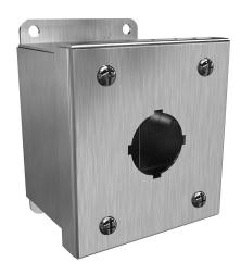
Hammond pushbutton enclosure, 1 hole, 30mm, NEMA 3R/4/4X, 4 x 4 x 3in (HxWxD), wall mount, 316 stainless steel, #4 brush finish, screw cover.
