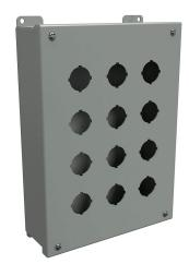
Hammond pushbutton enclosure, 12 holes, 30mm, NEMA 12/13, 12 x 9 x 3in (HxWxD), wall mount, carbon steel, ANSI 61 gray, powder coat finish, hinged screw cover.
