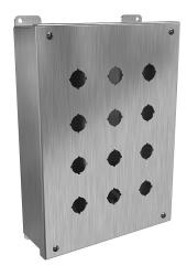
Hammond pushbutton enclosure, 12 holes, 22mm, NEMA 3R/4/4X, 12 x 9 x 3in (HxWxD), wall mount, 304 stainless steel, #4 brush finish, hinged screw cover.
