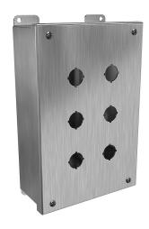
Hammond pushbutton enclosure, 6 holes, 22mm, NEMA 3R/4/4X,  $10 \times 7 \times 3$ in (HxWxD), wall mount, 304 stainless steel, #4 brush finish, hinged screw cover.
