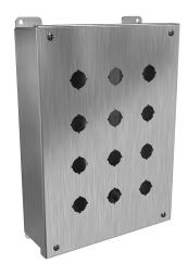
Hammond pushbutton enclosure, 12 holes, 22mm, NEMA 3R/4/4X, 12 x 9 x 3in (HxWxD), wall mount, 316 stainless steel, #4 brush finish, hinged screw cover.
