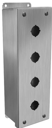
Hammond pushbutton enclosure, 4 holes, 22mm, NEMA 3R/4/4X, 11 x 4 x 3in (HxWxD), wall mount, 316 stainless steel, #4 brush finish, screw cover.
