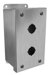
Hammond pushbutton enclosure, 2 holes, 22mm, NEMA 3R/4/4X, 6 x 4 x 3in (HxWxD), wall mount, 316 stainless steel, #4 brush finish, screw cover.
