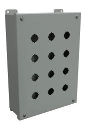
Hammond pushbutton enclosure, 12 holes, 22mm, NEMA 12/13, 12 x 9 x 3in (HxWxD), wall mount, carbon steel, ANSI 61 gray, powder coat finish, hinged screw cover.
