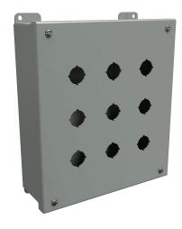
Hammond pushbutton enclosure, 9 holes, 22mm, NEMA 12/13, 10 x 9 x 3in (HxWxD), wall mount, carbon steel, ANSI 61 gray, powder coat finish, hinged screw cover.
