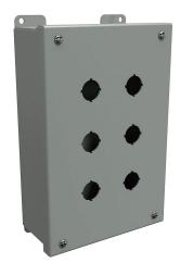
Hammond pushbutton enclosure, 6 holes, 22mm, NEMA 12/13,  $10 \times 7 \times 3$  in (HxWxD), wall mount, carbon steel, ANSI 61 gray, powder coat finish, hinged screw cover.
