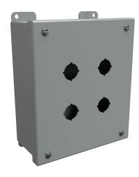
Hammond pushbutton enclosure, 4 holes, 22mm, NEMA 12/13, 8 x 7 x 3in (HxWxD), wall mount, carbon steel, ANSI 61 gray, powder coat finish, hinged screw cover.
