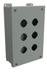
Hammond pushbutton enclosure, 6 holes, 30mm, NEMA 12/13, 10 x 7 x 3in (HxWxD), wall mount, carbon steel, ANSI 61 gray, powder coat finish, hinged screw cover.
