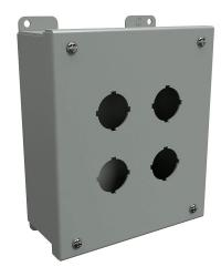
Hammond pushbutton enclosure, 4 holes, 30mm, NEMA 12/13, 8 x 7 x 3in (HxWxD), wall mount, carbon steel, ANSI 61 gray, powder coat finish, hinged screw cover.
