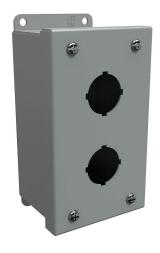
Hammond pushbutton enclosure, 2 holes, 30mm, NEMA 12/13, 6 x 4 x 3in (HxWxD), wall mount, carbon steel, ANSI 61 gray, powder coat finish, screw cover.
