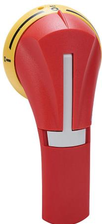
Socomec rotary handle, pistol, S2, red/yellow, external front mount, 3-position, lockable in OFF only, defeatable, NEMA 4/4X. For use with SIRCOVER transfer switch bodies.
