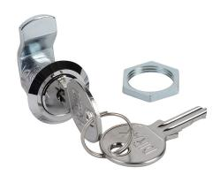
Hammond enclosure latch, keylocking, 1/4-turn flush-mount, 1-point, plated steel, chrome finish. For use with 1420 and N1A enclosures. (2) keys included.
