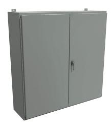
Hammond enclosure, NEMA 12, 48 x 48 x 12in (HxWxD), wall mount, carbon steel, ANSI 61 gray, powder coat finish, doubledoor, 3-point keylocking handle.
