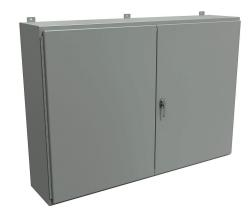
Hammond enclosure, NEMA 12, 42 x 60 x 12in (HxWxD), wall mount, carbon steel, ANSI 61 gray, powder coat finish, doubledoor, 3-point keylocking handle.
