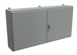
Hammond enclosure, NEMA 12, 30 x 60 x 10in (HxWxD), wall mount, carbon steel, ANSI 61 gray, powder coat finish, doubledoor, 3-point keylocking handle.
