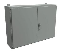
Hammond enclosure, NEMA 12, 30 x 42 x 10in (HxWxD), wall mount, carbon steel, ANSI 61 gray, powder coat finish, doubledoor, 3-point keylocking handle.
