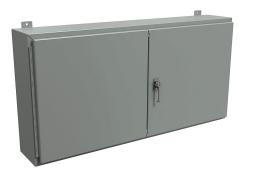
Hammond enclosure, NEMA 12, 24 x 48 x 8in (HxWxD), wall mount, carbon steel, ANSI 61 gray, powder coat finish, double-door, 3-point keylocking handle.
