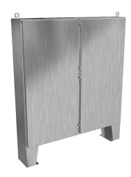
Hammond enclosure, NEMA 3R/4/4X/12/13, 72 x 72 x 12in (HxWxD), floor mount, 304 stainless steel, #4 brush finish, 2-door, stainless steel clamps, padlock hasp and staple.
