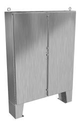
Hammond enclosure, NEMA 3R/4/4X/12/13, 72 x 60 x 12in (HxWxD), floor mount, 304 stainless steel, #4 brush finish, 2-door, stainless steel clamps, padlock hasp and staple.
