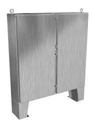
Hammond enclosure, NEMA 3R/4/4X/12/13, 60 x 60 x 12in (HxWxD), floor mount, 304 stainless steel, #4 brush finish, 2-door, stainless steel clamps, padlock hasp and staple.
